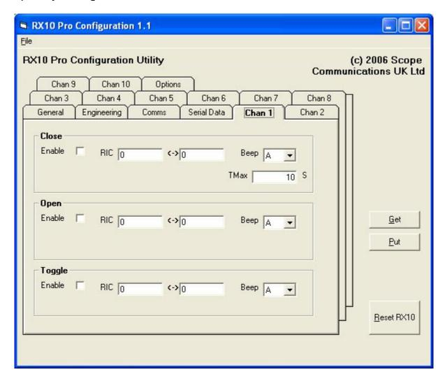
Each relay can be controlled using a range of RIC's to close, open or toggle the state of the relay.
