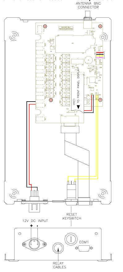
Note! When re-fitting the front panel ribbon cable, ensure that the connector collar is raised and check that the cable is square to the connector. Ensure that the cable runs straight in the direction shown. Gently insert the cable tail as far as it will go, then push down equally on both sides of the connector collar.
