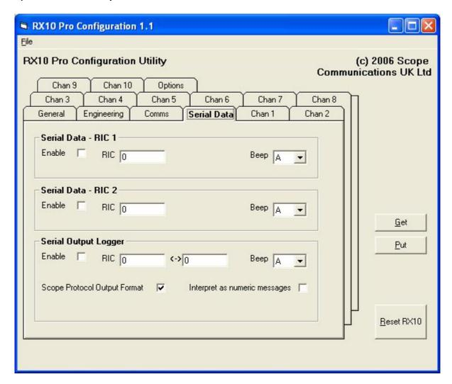
Where it is required to send message data for onward transmission or for logging purposes, the serial port can be enabled. The RX10 can be programmed to accept either two individual RIC's or a range of RIC's. Note: the RX10 does not provide time/date stamping, although this function could be facilitated using suitable software on a PC, or by using a POS style printer with an onboard real time clock.
