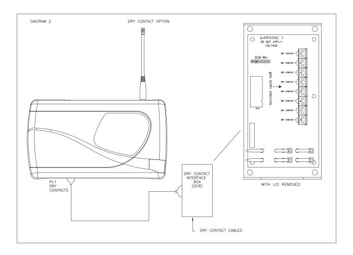
This option must be specified at time of ordering, along with the pre-programmed messages required. The purchaser should also order the dry contact interface box (Part Code: DC8) for ease of connection to the contact terminals (see Diagram 2).
